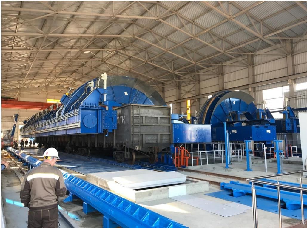
Technical innovation in Taman Seaport: Two SCHADE Wagon Tippers working in parallel each unload three wagons fully loaded with coal - 60 wagons each per hour (Photo SCHADE).
