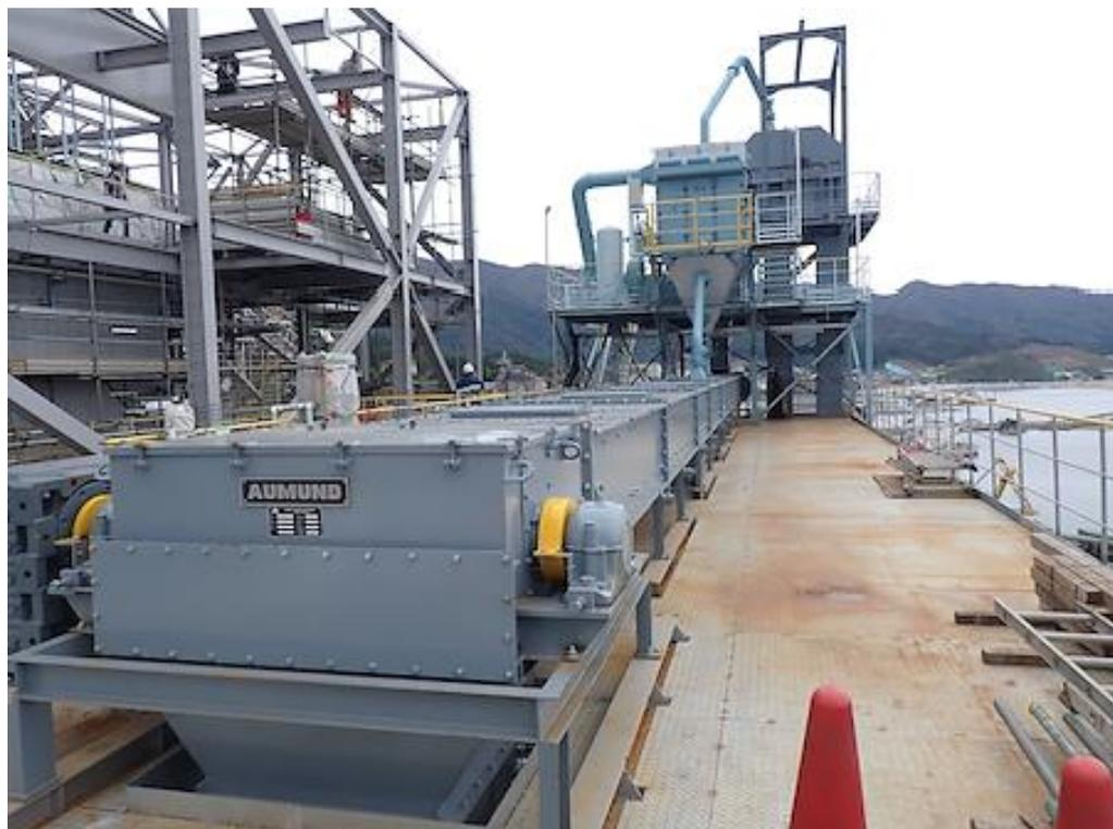
AUMUND Drag Chain Conveyor type LOUISE TKF for handling alternative fuels in Taiheiyo Cement's Ofunato Power Plant in Iwate Prefecture, Japan (© AUMUND)
