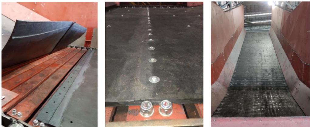
The belt is connected to the apron bars
