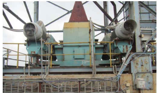
Deep Pan Conveyor feeding Cement Mill Hopper
